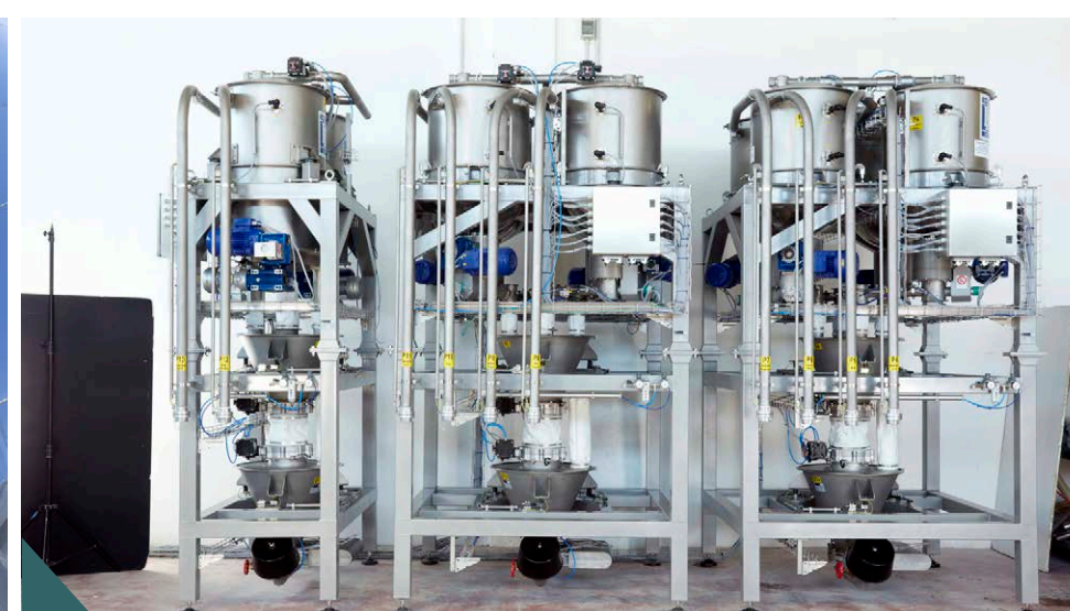
Series or star groups for volumetric micro-dosages of powder, granule, solid and liquid ingredients
